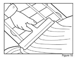
To further improve the adhesive qualities the floor can be primed once more using undiluted primer, the matting will then bond very well to the floor. The mesh can also be stapled to plasterboards.
