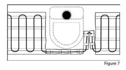
Cut and release a piece of mesh and go round toilets and the like. Cut another piece of mesh and place the cable as shown in the figure. Now, the matting can be rolled out at the right side, otherwise the installation will be more difficult (Figure 7).
